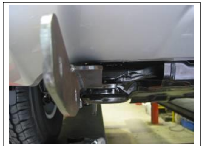
Figure 4: ECB Steel mounting brackets fitted
