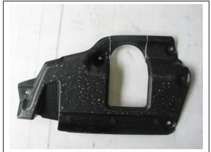
Figure 2: Under body trim cut lines
