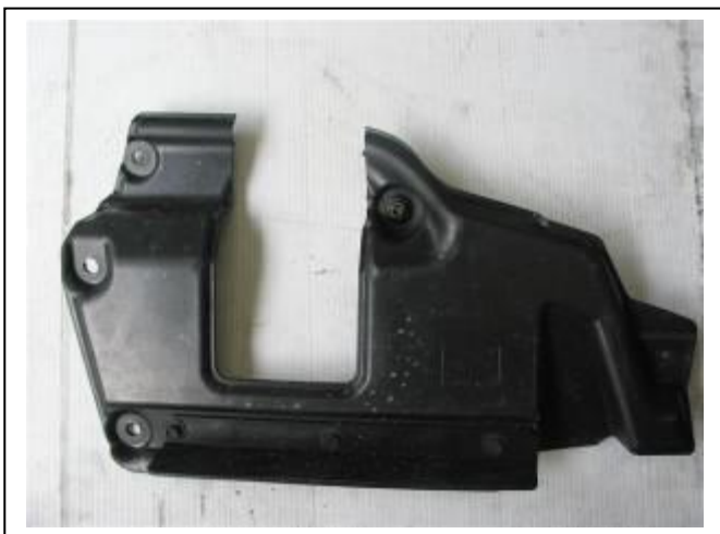
Figure 3: Trimmed under body shields.
